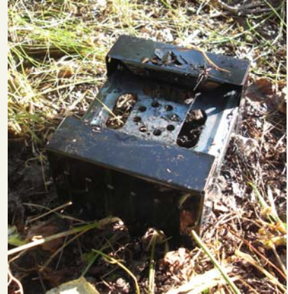
This little 'Fold-a-Stove' was an experiment, and Cindy ended up really liking it. You fuel it with a single pellet in the middle. It is tiny, folds up compact with the pellets inside, and only cost $5.99 at Army/Navy Store. It took one pellet to fry potatoes and 2-3 to boil water.
